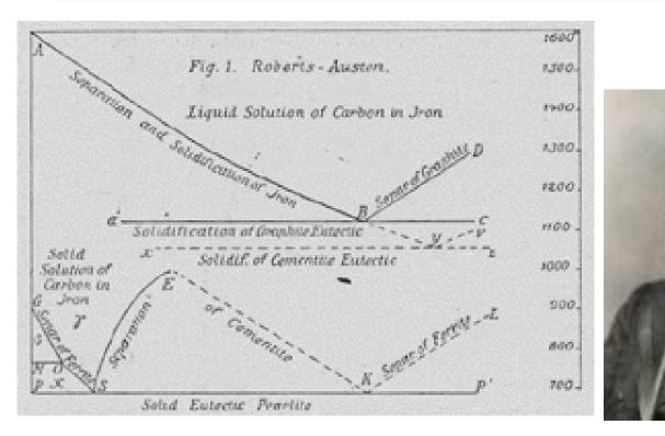
Initial work on the most crucial phase diagram in metallurgy lays the foundation for an indispensable tool in many other material systems.
