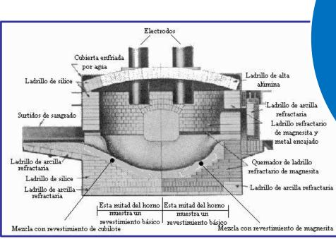
The predecessor of the modern electric arc furnace, which is the foundation of modern steel production and many other alloys.
