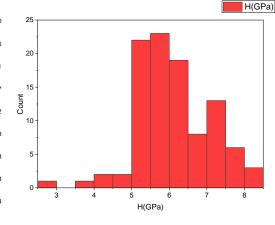
The effect of chemistry on nanohardness distribution in Q&P treated steels. Left: EBSD phase map, analyzed area, relevant nanohardness distribution map and histogram of nanohardness distribution for a low alloyed steel; Right: for a highly alloyed steel.
