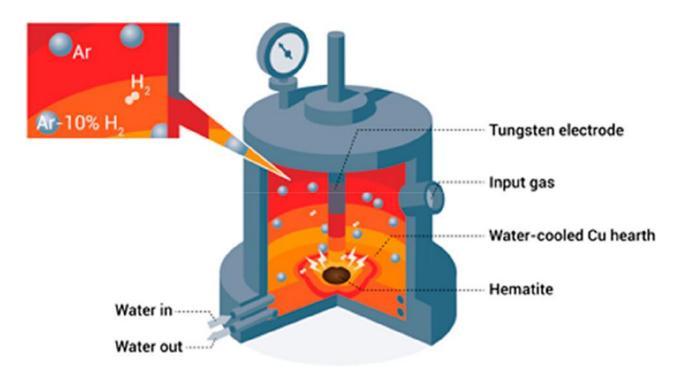
Experimental setup for hydrogen-plasma-based smelting reduction of iron oxides with a process using a 10% H2–90% Ar gas mixture to produce the plasma.
