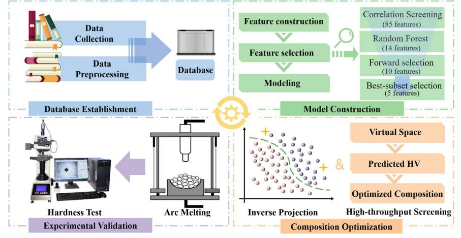
Diagram of machine learning-based alloy design system for the HEAs with desired hardness.
