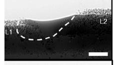
Melt pool Sintered powder L5 L4 L3 Lack of fusion
