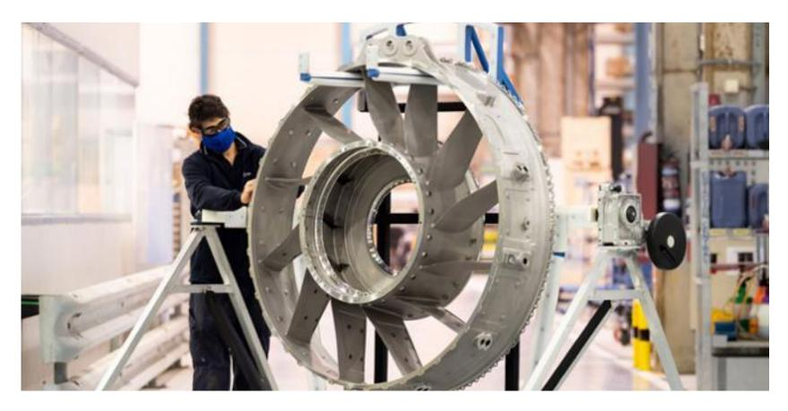
ITP Aero desingn and manufacture a main structure of a new airplane engine UltraFan® through SLM 19/10/2021
