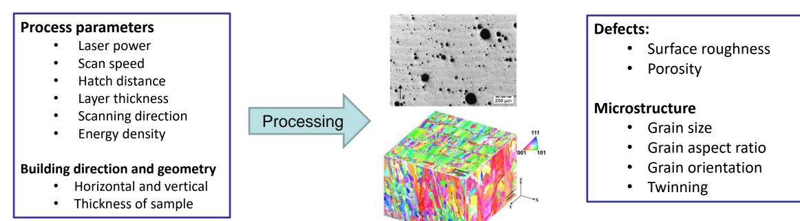
If the SLM resulting microstructure is given (experimentally or predicted by virtual testing), is it posible to predict the macroscopic response?
